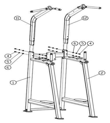
**Illustration**: Shows how to attach the extension frames (#11 and #12) to the uprights (#1 and #2) using screws (#4), spring washers (#5), and flat washers (#6).
