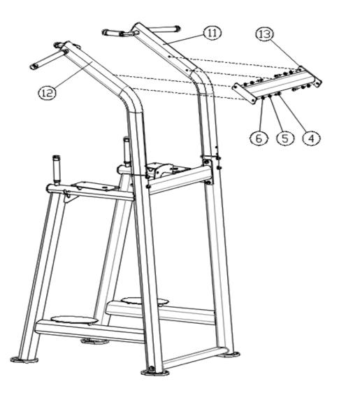
**Illustration**: Shows how to mount the connector frame (#13) at the top between the two vertical extension frames (#11 and #12). Use screws (#4), spring washers (#5), and flat washers (#6) as shown.
