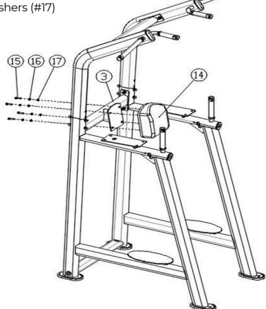
**Illustration**: Shows how to mount the back pad (#14) onto the upper frame bracket (#3) using screws (#15), spring washers (#16), and flat washers (#17).
